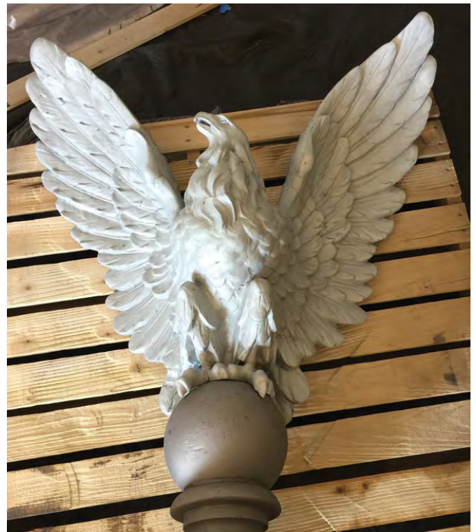
Figure 16. Aluminum is a highly corrosion-resistant metal that is commonly used as a substitute material for cast iron. Aluminum can be a more affordable and lightweight alternative to cast iron that retains a similar texture, shape, and maintenance cycle. Photo: NPS.
