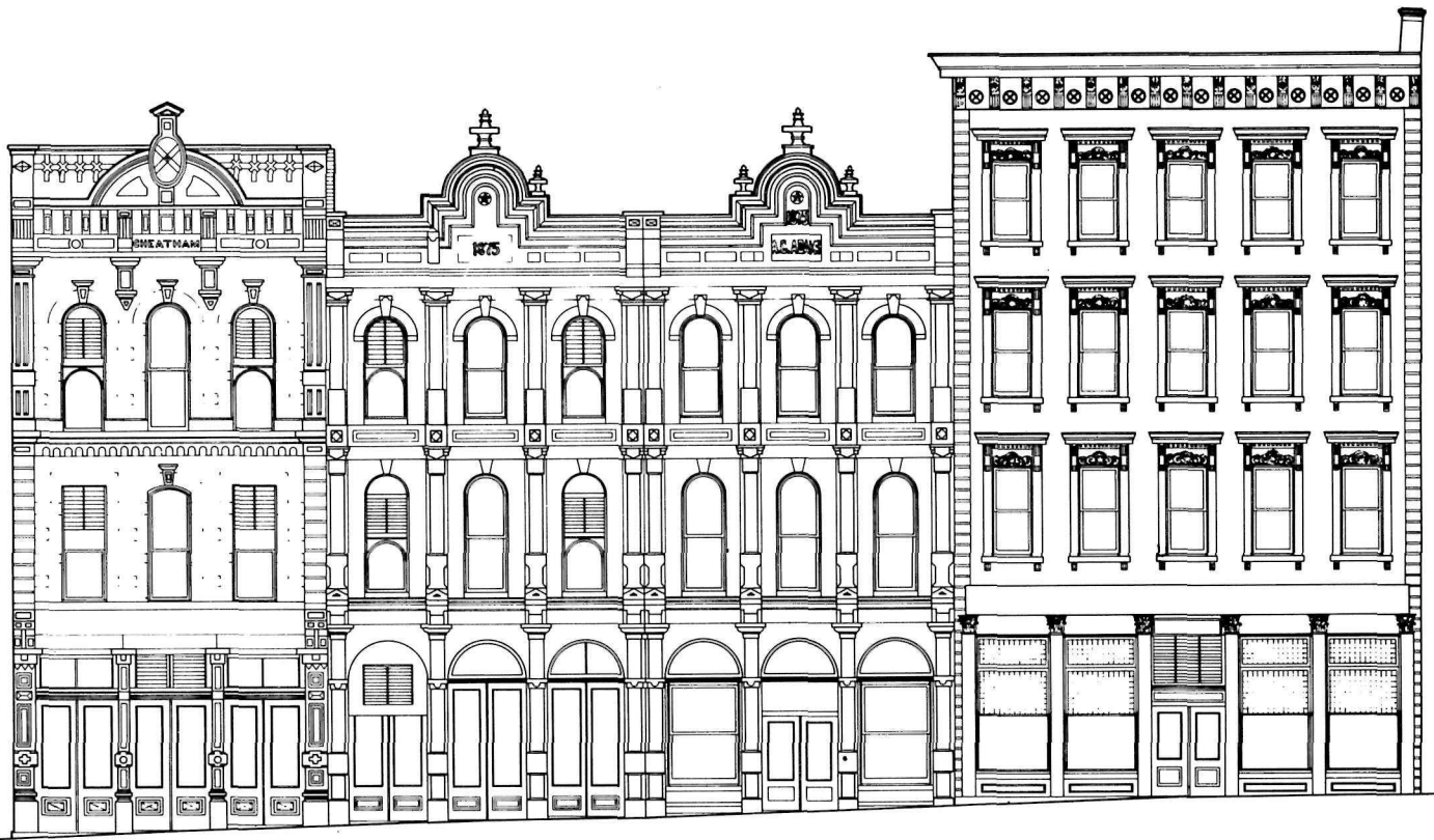
These Victorian storefronts on the Public Square in Nashville, Tenn., vary in design, but the similarities in their materials, scale, and proportions produce an overall unity. Cast iron was used for the cornices and the pilasters which divide the ground floor bays. TENN-16, sheet 3
