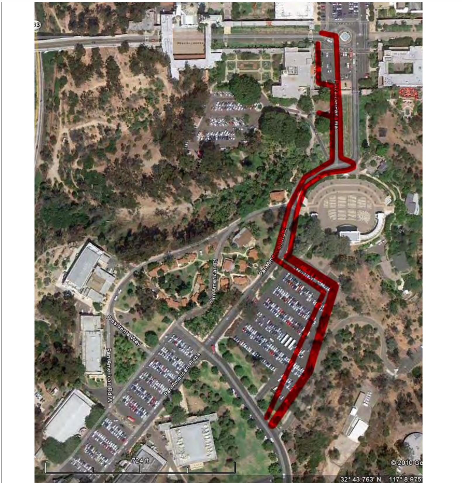
Figure A-7 – Modified SOHO Plan with features of the Plaza de Panama Committee Plan showing two-way access through the Plaza de California, El Prado, the southwest corner of the Plaza de Panama, the west Esplanade, and portions of Pan American Road. Including a new vehicular traffic circulation pattern and two way lanes behind the Spreckles Organ Pavilion, moving through-traffic to the east side of the existing parking lot. Thus eliminating “the traffic congestion at the intersection of Pan American Road and Presidents Way, and shifting the vehicular interchange to the east, the current intersection is abandoned allowing for the future removal of parking from Pan American Plaza.”
