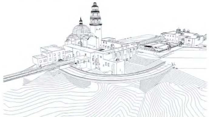
Image 18: Conceptual bird's eye rendering, looking northeast, showing the bypass bridge and related abutments. This drawing shows the general size and location of the bridge, but the design has not been completed or refined.
